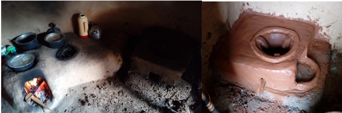
Figure 3: A typical jiko used by the community and a completed improved kuni mbili jiko
